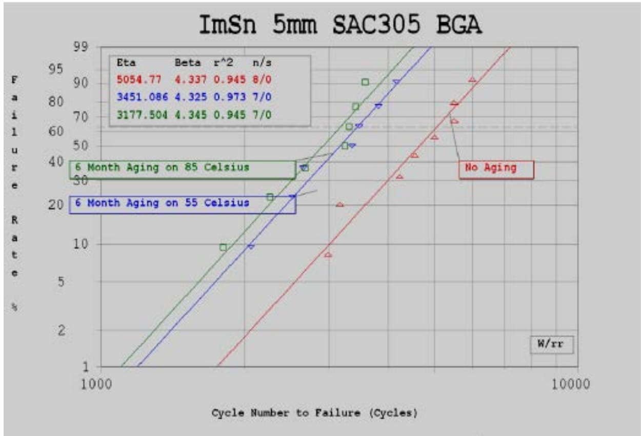
Figure 3: SAC 305 on ImSn for 5mm BGA [Hai 2013]
