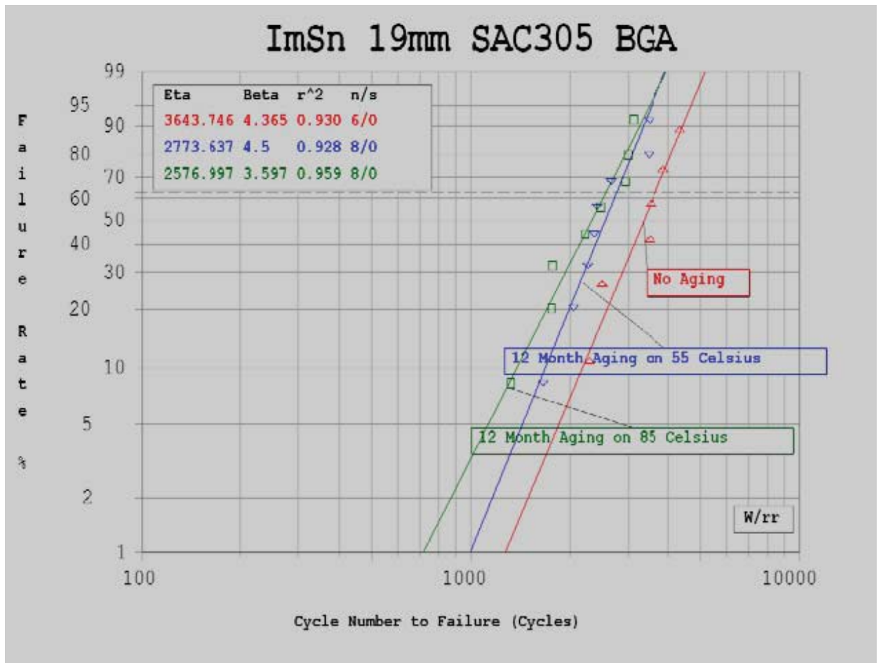
Figure 8: SAC 305 on ImSn for 19mm BGA [Hai 2013]
