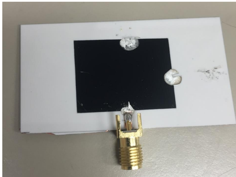
Figure 5.3 2.4 GHz Carbon Nanotube Patch Antenna
