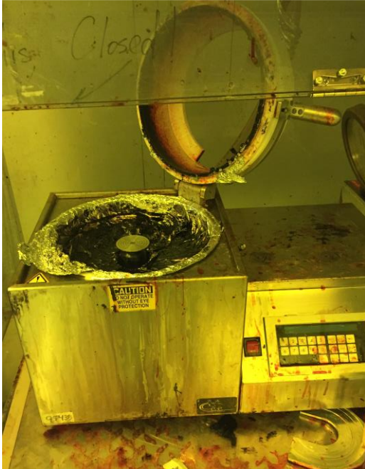
Figure 3.4 (Left) Spinner to apply photoresist. (Right) Heater for the soft bake
