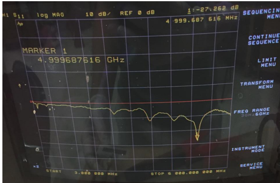
Figure 5.7 S11 Measurement for the 5 GHz Patch Antenna
