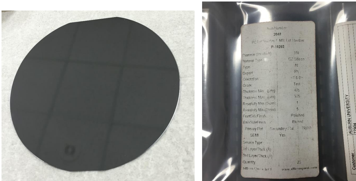
Figure 3.1 (Left) N-type Silicon wafer. (Right) Wafer details from packaging.
