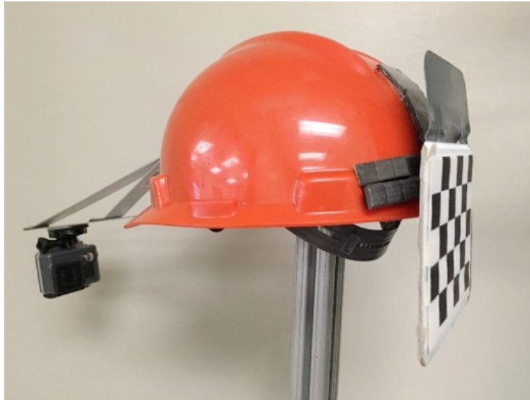
Figure B.1: Hard hat designed for tracking gaze and head motion
