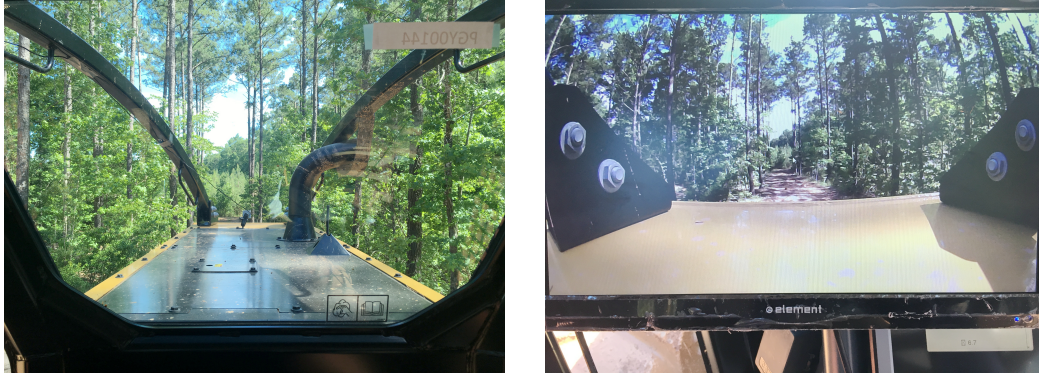
Figure 5.3: Vision comparison between driver's vision and live video
