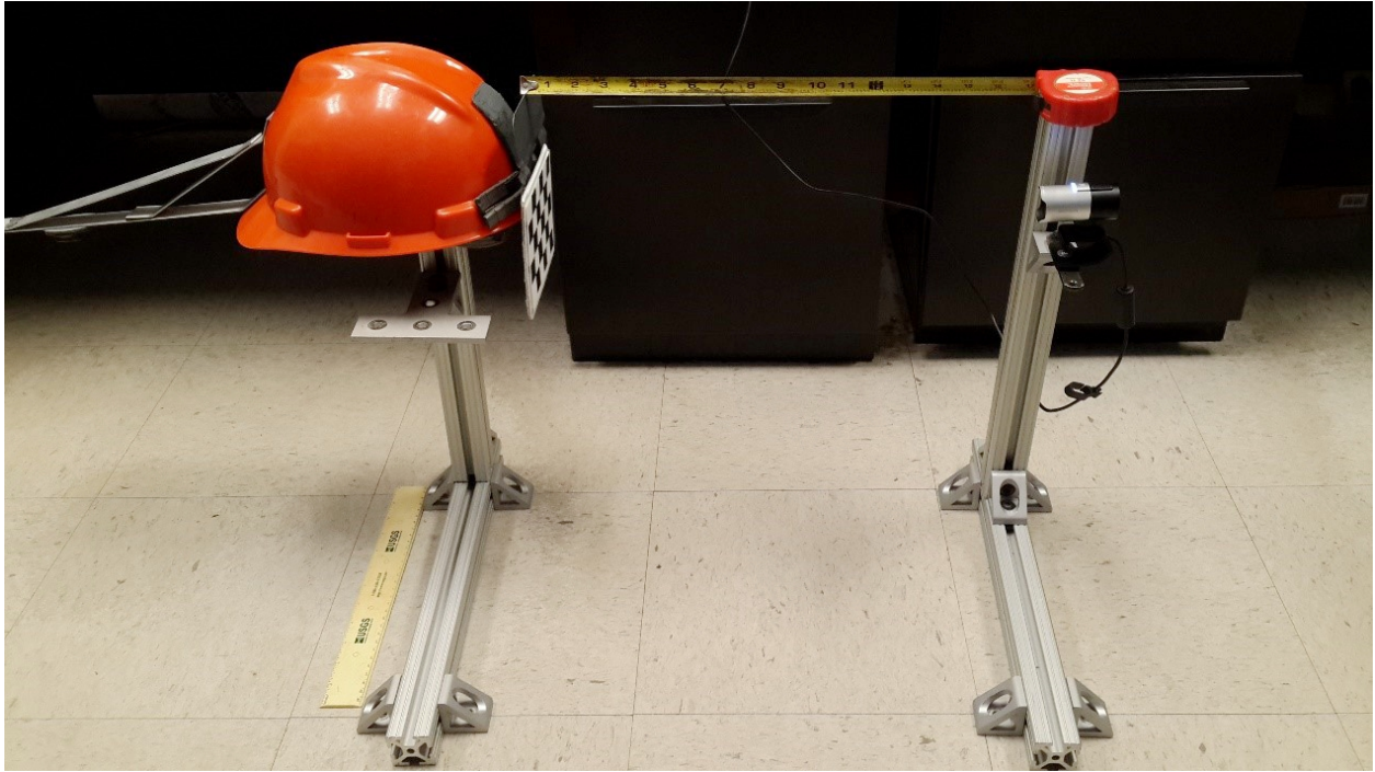
Figure 3.18: Calibration of pose estimation
