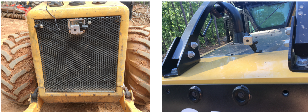
Figure 5.2: Fisheye camera set on the front of both skidders
