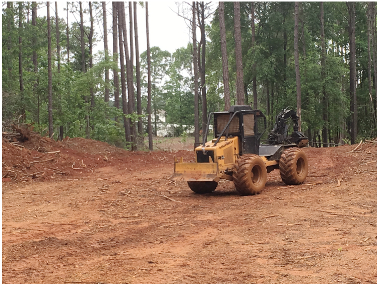
Figure B.3: TurboForest mini skidder with windows covered during driving tests
