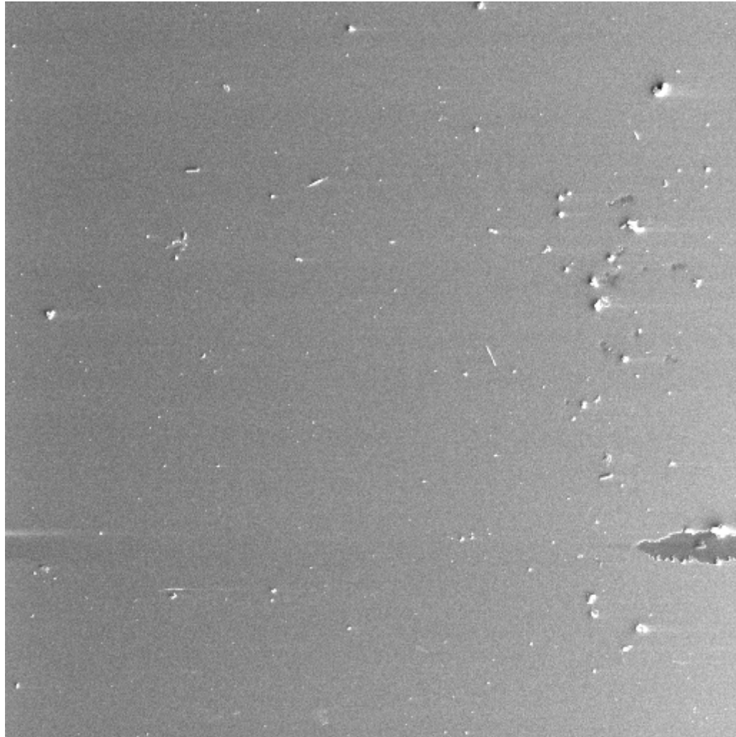
Figure 3.2 Control experiment: SEM image (500×) of captured Salmonella enterica Typhimurium on butanethiol SAMs pretreated with anti- Salmonella antibody solution
