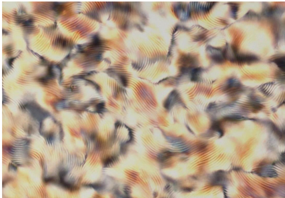
Figure 4.13 Enlarged region of Figure 4.12f showing the cholesteric fingerprint texture. Scale bar is 100 \mu\text{m} .
