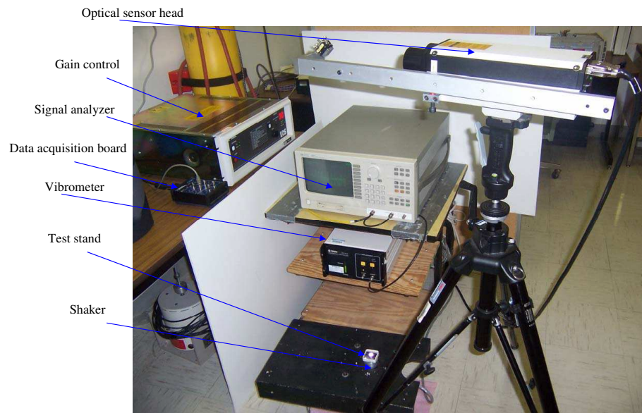
Figure 5.6: Photograph illustrates the experimental setup with the laser displacement measurement system
