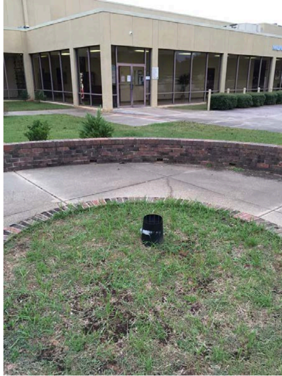
Figure 2.10: Rain gauge installed at the Prichard Municipality complex
