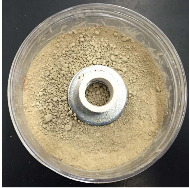
Figure 70: SWCC Specimen with Washer and PVC Pipe Piece
