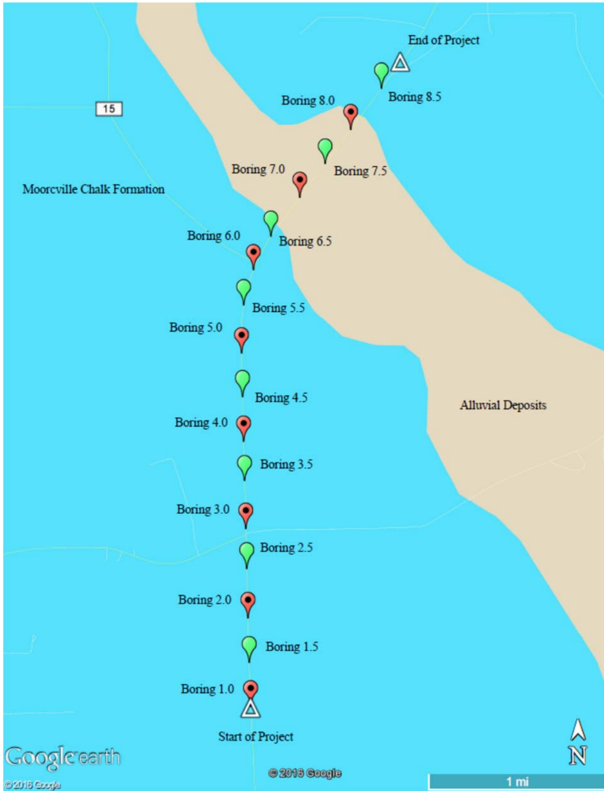
Figure 29: Google Map of Alabama Highway 5 (Google Earth 2014) overlaid with USGS Soil Survey Map (Szabo et al. 1988)
