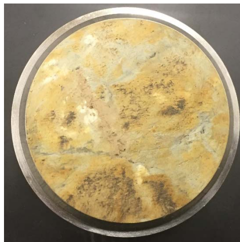
Figure 55: Prepared Swell Test Specimen
