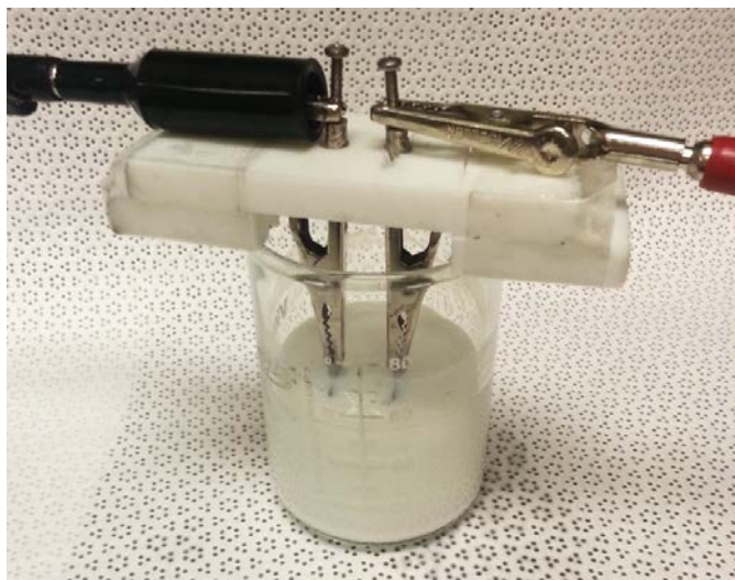
Figure 12. The deposition cell of the EPD process
