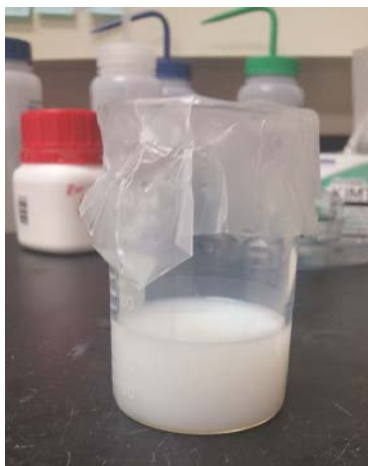
Figure 10. ZnO in ethanol suspension with concentration of 0.02 g/ml.
