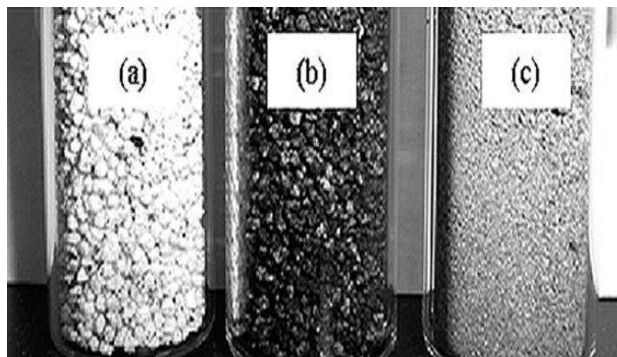
Figure 3.1. Macroscale appearance of PP-SWNT after initial mixing but before melt extrusion for (a) dry mixing, (b) rotary evaporation, and (c) hot coagulation [25].
