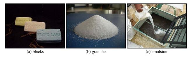
Figure 2.3 PAM Types (Applied Polymer Systems Inc. 2016).
