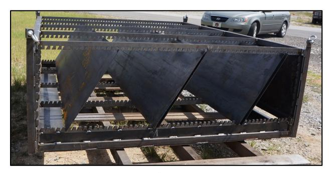
Figure 4.22 Lamella Settler Unit without Plates.
