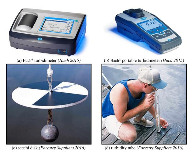
Figure 2.9 Turbidity Measuring Apparatus.
