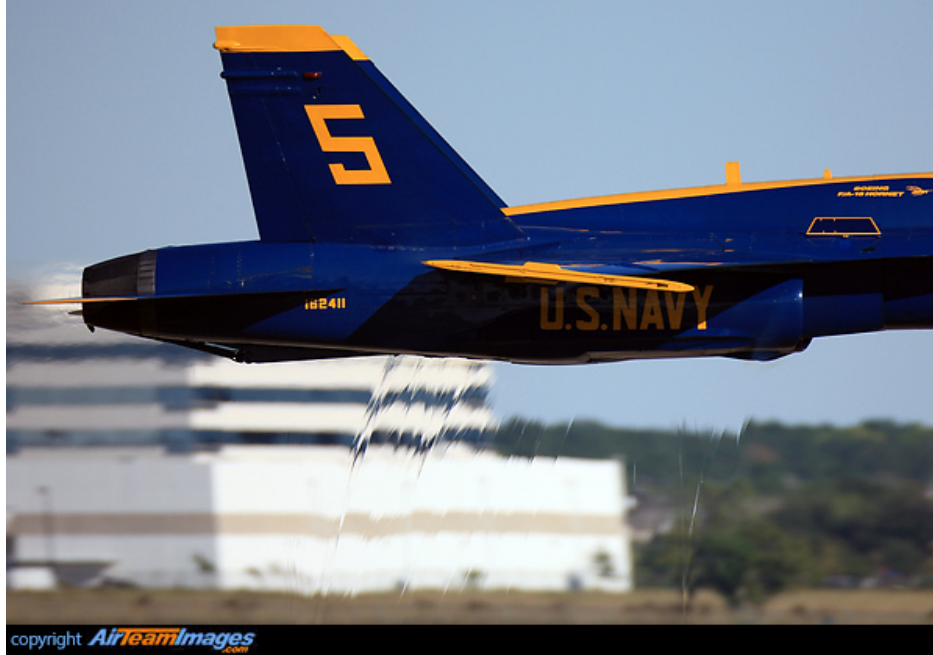
Figure 2.5: A Blue Angel F/A-18 Hornet [1] distorting the background during flight shows the same concept that the BOS technique exploits during an experiment.
