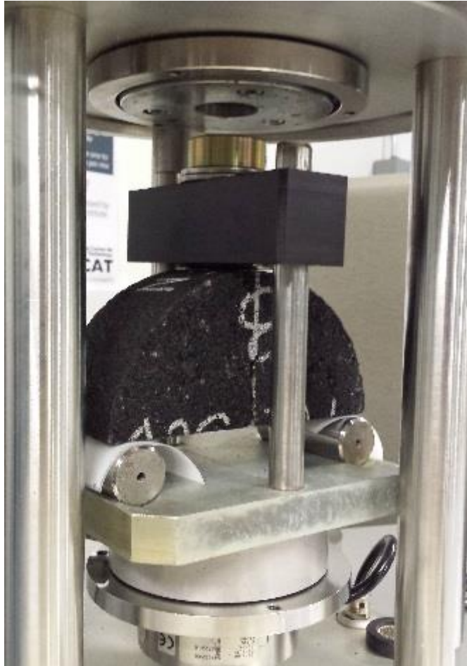
Figure 17. SCB-LTRC test setup using an AMPT.
