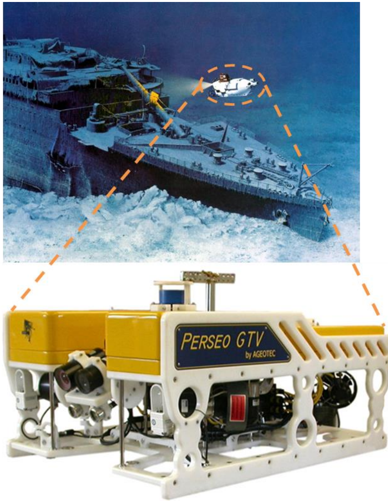
Figure 1.1: Photograph of marine exploration device shown to explore the Titanic wreckage (top) (ref: http://ultimatetitanic.com/the-wreckage/#.U0cDgvldXTo ). Photograph of similar marine exploration device “Perseo GTV” made of syntactic foam (bottom) (ref: http://www.diabgroup.com/en-GB/About-us/This-is-DIAB )
