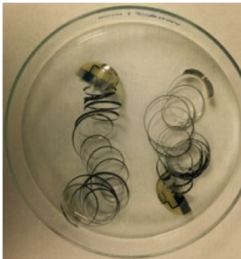
Figure 3.13: A set of 1 meter long stripline flex cables released from a 125 mm diameter Si wafer.
