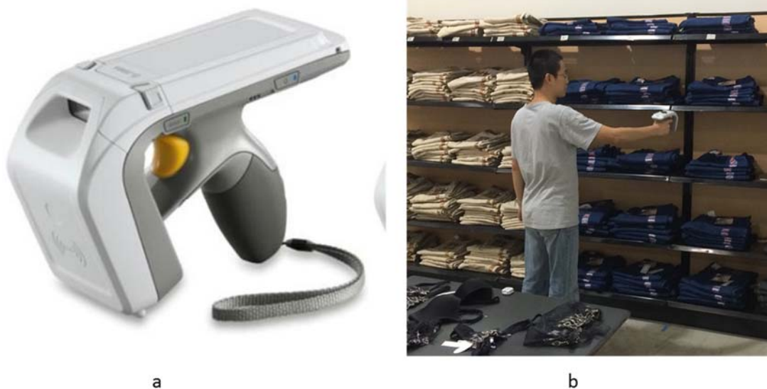
Figure 6.11(a) Zebra RFD8500 handheld, (b) waving handheld in front of merchandise to do manual inventory.
