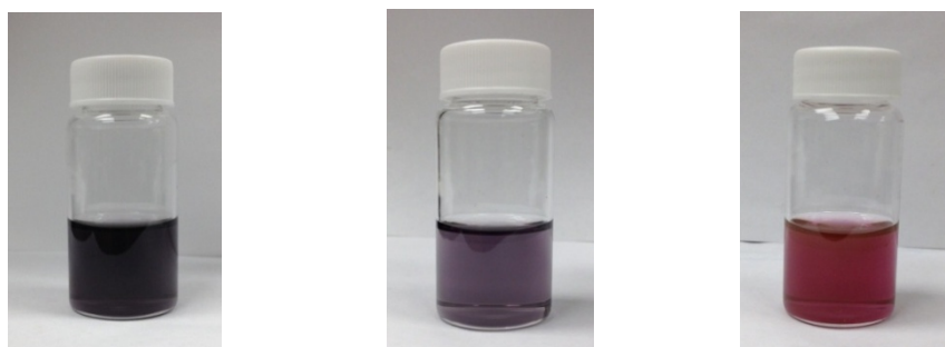
Figure 2.5: Au nanoparticles as prepared (left) and after dilution (2 times) (middle) and without SH-NDI-DPA (right).
