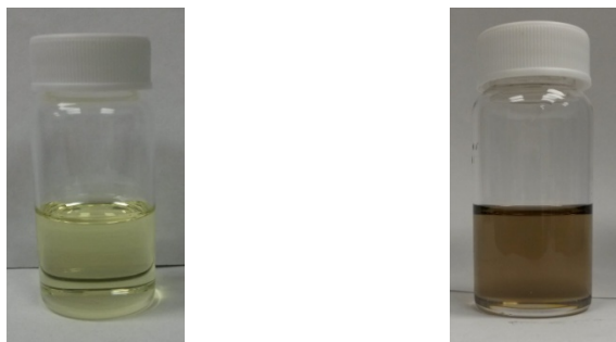
Figure 5.1: CdS nanoparticles (2 mM) in the reaction mixture without DPA-NDI-SH (left) and with DPA-NDI-SH (right).
