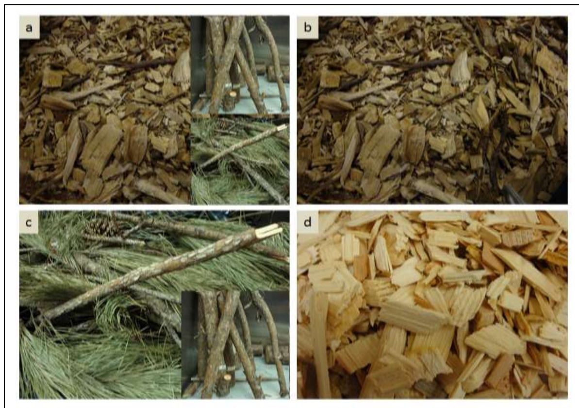
Figure 5.1: Loblolly pine logging residues: (a) whole, (b) wood & bark, (c) slash and (d) wood.
