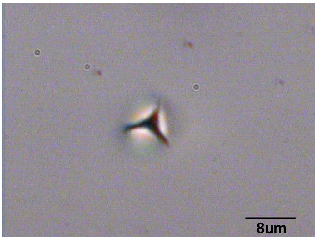
Figure 4.21 NFC film pile-up after nanoindentation test
