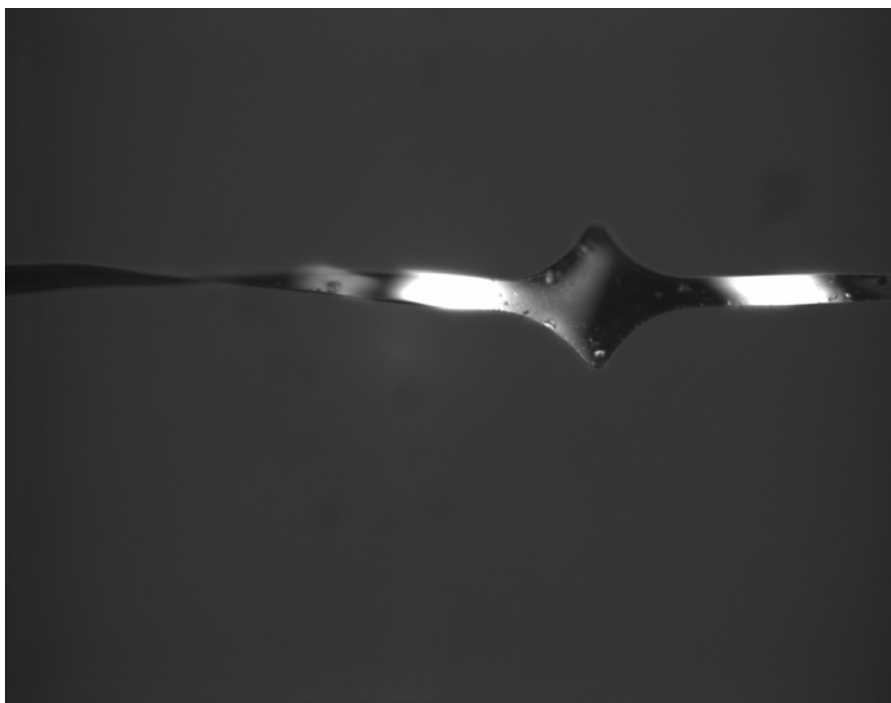
Figure 4.6b Image of the membrane twisting during H_3PO_4 etching (Nikon Microscope 50x)
