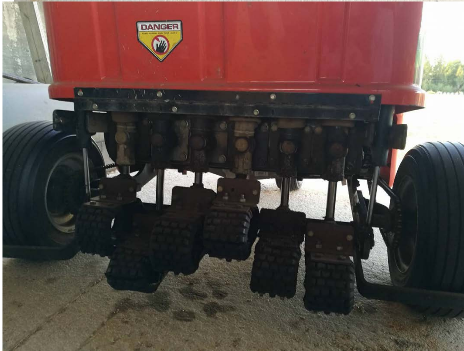
Figure 1. The Cady traffic simulator unit, used to apply artificial traffic in Experiments 1 and 3.
