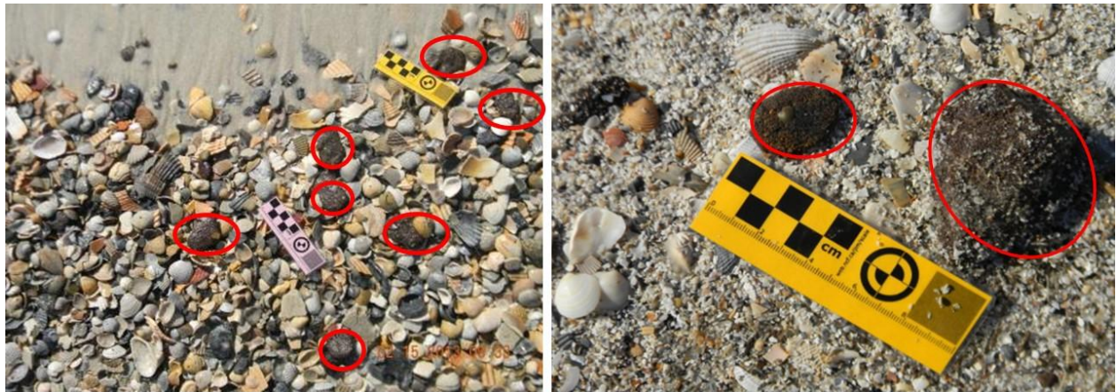
Figure 2-12. Surface residual balls (SRBs) indicated by red circles that are deposited with shells on a beach following the Deepwater Horizon oil spill
