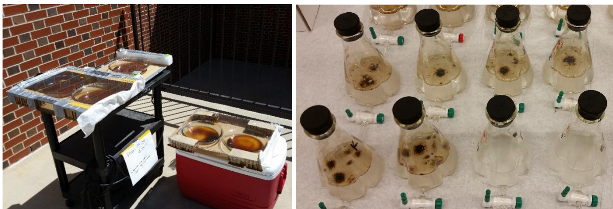
Figure 3-1. Experimental methods: Left) outdoor oil weathering method; Right) baffled flask experiments
