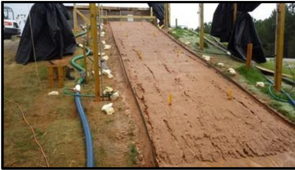
(e) slope erosion after interval 4
