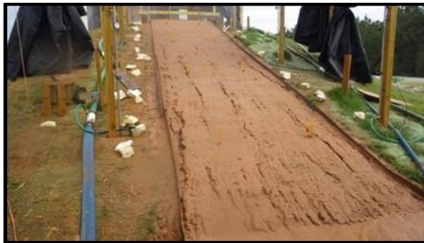
(g) slope erosion after interval 6
