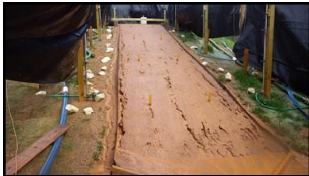
(e) slope erosion after interval 4
