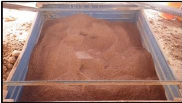
(c) screened soil stockpile
