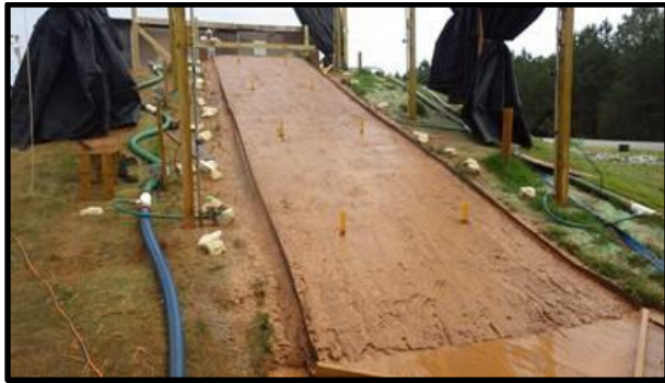
(c) slope erosion after interval 2
