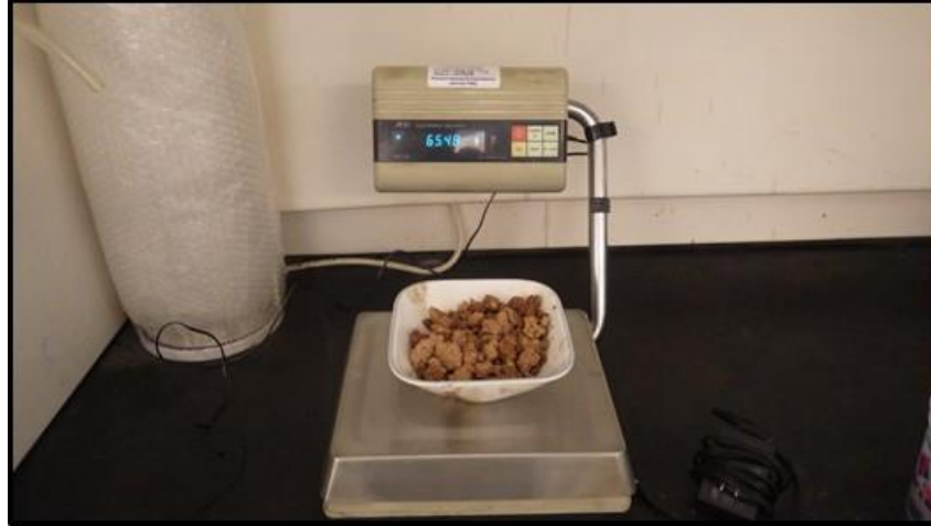
Figure 4.11 Drying Soil Using the Microwave Method.
