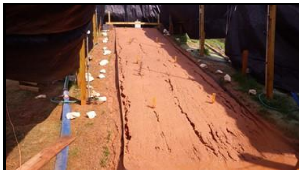
(g) slope erosion after interval 6
