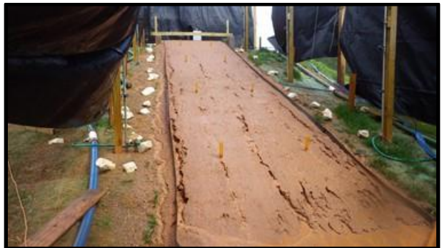
(f) slope erosion after interval 5
