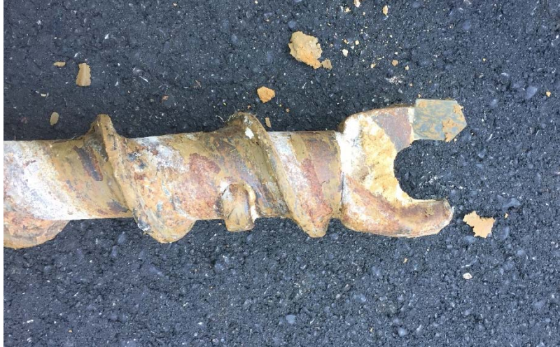
Figure 77: Auger and Bit used for Installation
