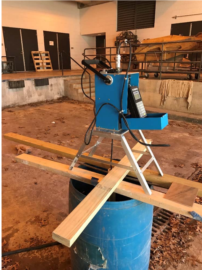
Figure 82: 55-Gallon Barrel Water Test Setup
