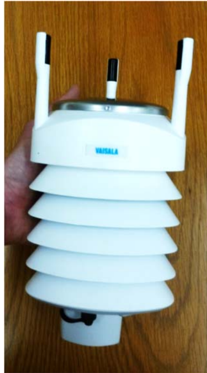
Figure 29: Campbell Scientific WTX520 Weather Sensor (Jackson 2016)
