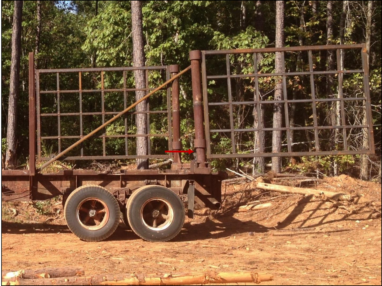
Figure 7. Constructed swinging gate modification.
