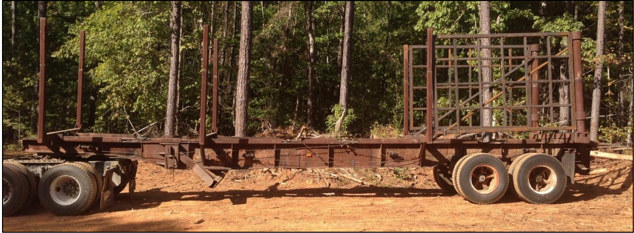
Figure 6. Donated trailer after alteration to a modern double bunk configuration.
