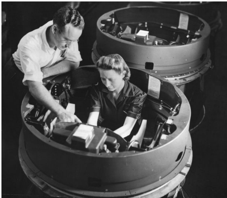
Fig. 2B.2: Assembling Emerson top aerial gun turret
