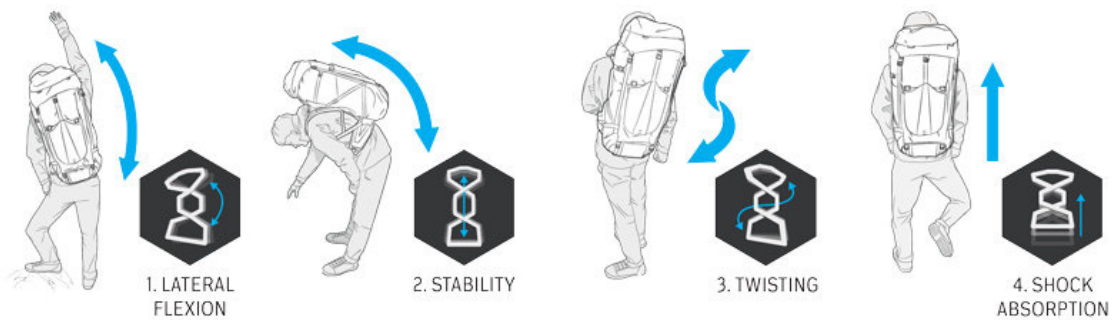
Fig. 4A.26: Movements of the Bergans carrier frame
