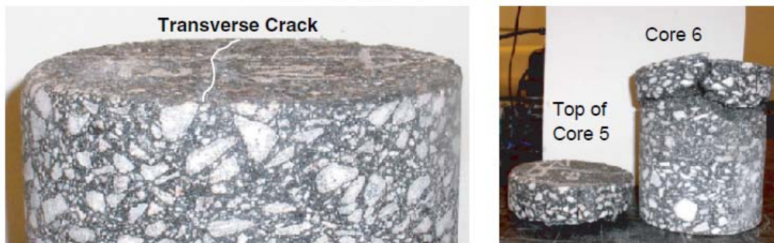
Figure 5.3- Cores from 2006-N1 showing TDC (Timm et al., 2009).
