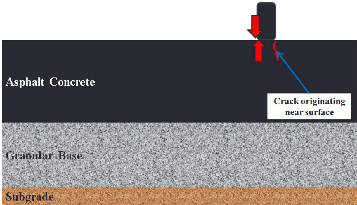
Figure 2.3 – TDC diagram with cracking due to shear stress at edge of tire.
