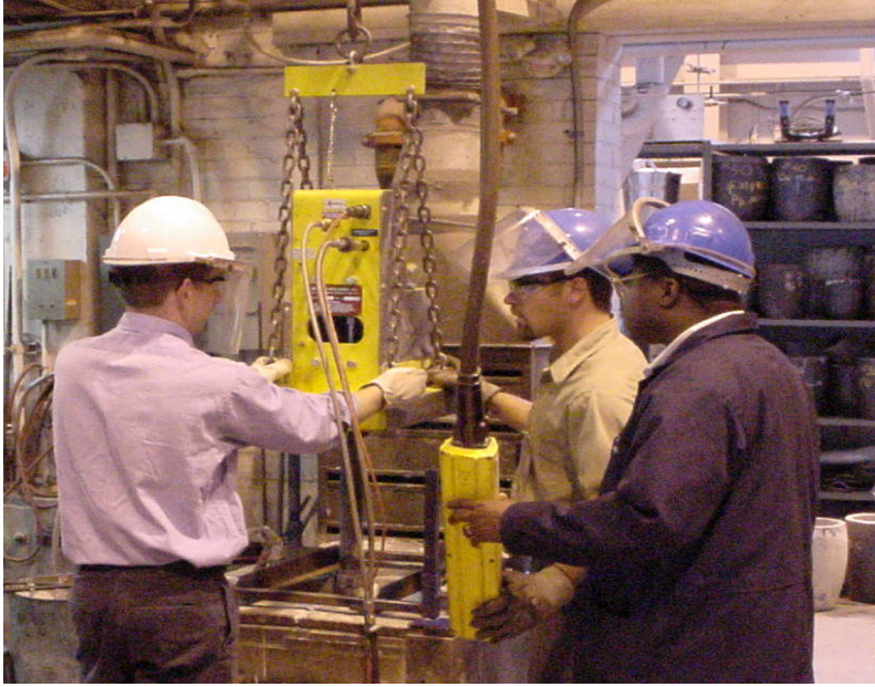
Figure 21 Commercial rotary degasser used to reduce hydrogen content in the melt between sensor measurements.
