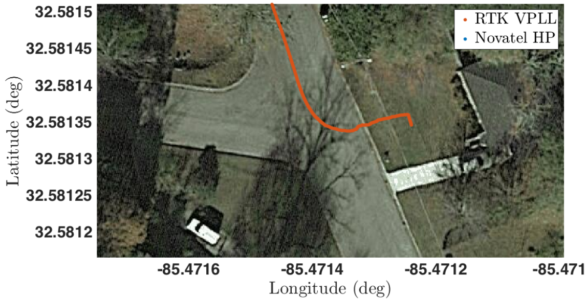
Figure 6.37: Despite difficulty of carrier phase tracking in the heavy foliage environment, the RTK VPLL algorithm provided a stable navigation solution with a bias of several meters in the final position estimates. The reference receiver was unable to calculate a high precision solution and is not seen in the figure. Imagery by Google, DigitalGlobe.
