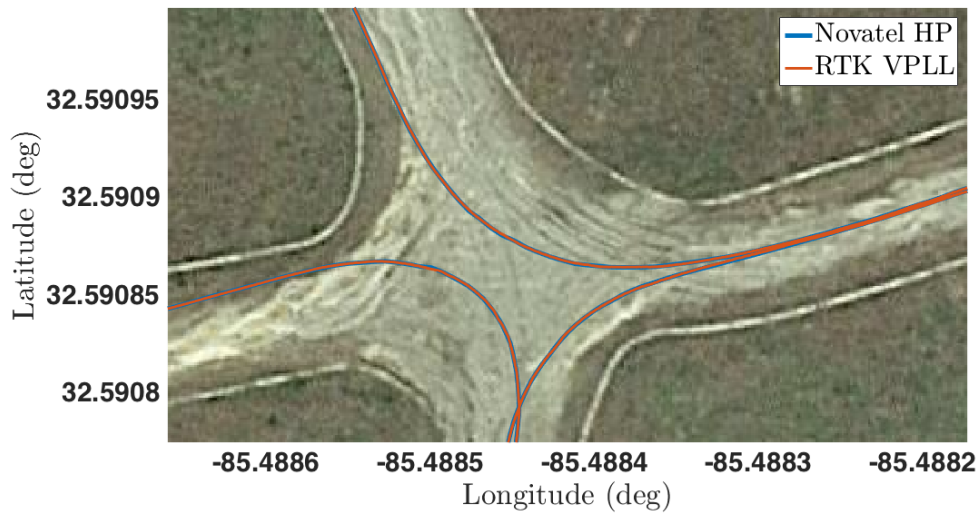
Figure 6.28: The RTK VPLL position and the reference RTK solutions are virtually identical in the image that shows the convergence of multiple laps. Imagery by Google, DigitalGlobe.
