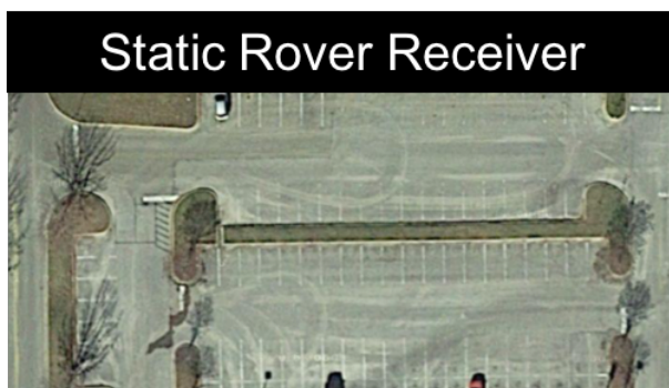
Figure C.4: The precision of the RTK solution was tested over a longer baseline (approximately 600 meters) using data from antenna positioned in a parking lot on the Auburn campus. Imagery by Google, DigitalGlobe.
