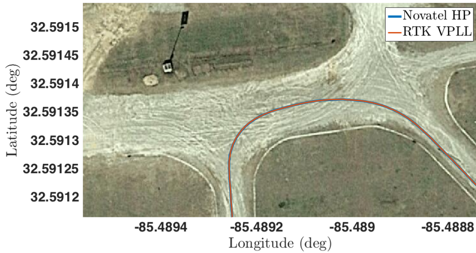
Figure 6.27: The RTK VPLL position solution is indistinguishable from the reference RTK solution in the first turn of the dynamic test. Imagery by Google, DigitalGlobe.
