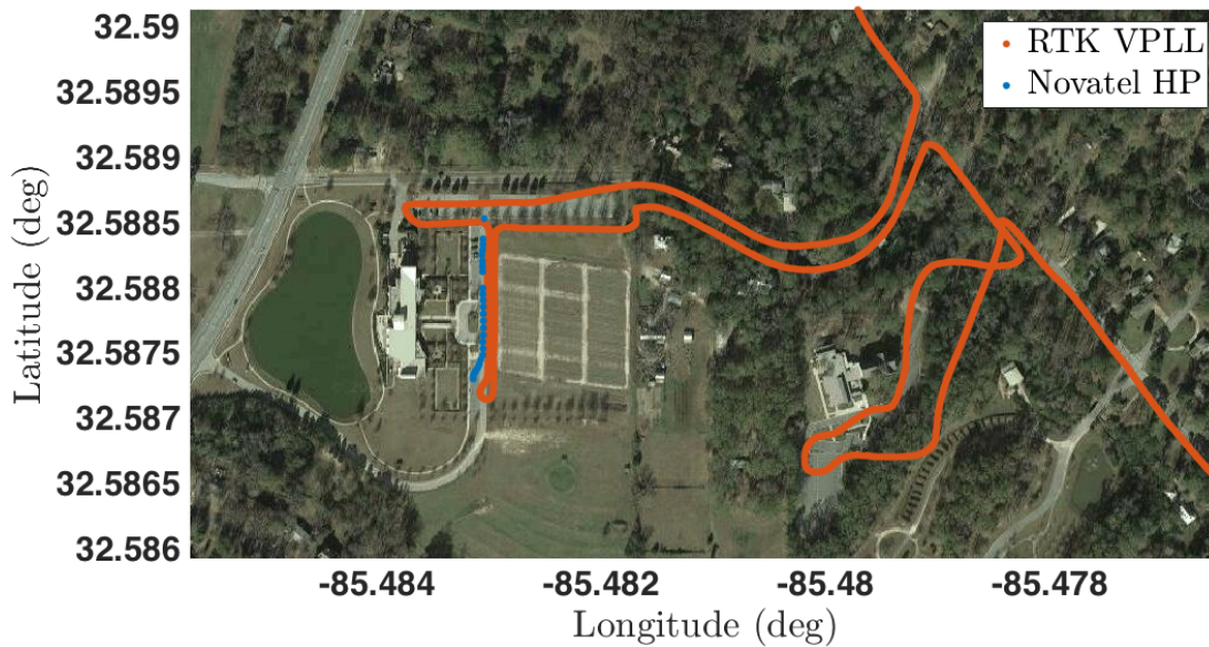
Figure 6.36: The RTK VPLL carrier phase tracking algorithm experience significant cycle slips in the most densely wooded areas. Imagery by Google, DigitalGlobe.
