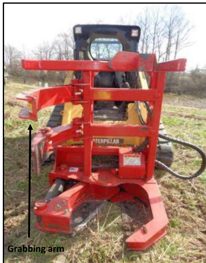
Figure 8: Fecon shear head with opened grabbing arm.
