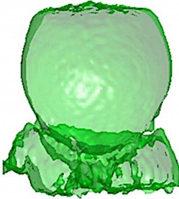
Figure 26 2D Solder Ball Lifting
