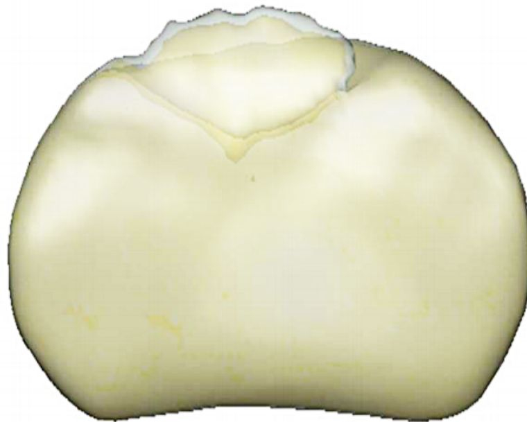
Figure 19 3D Reconstruction of Solder Crack
