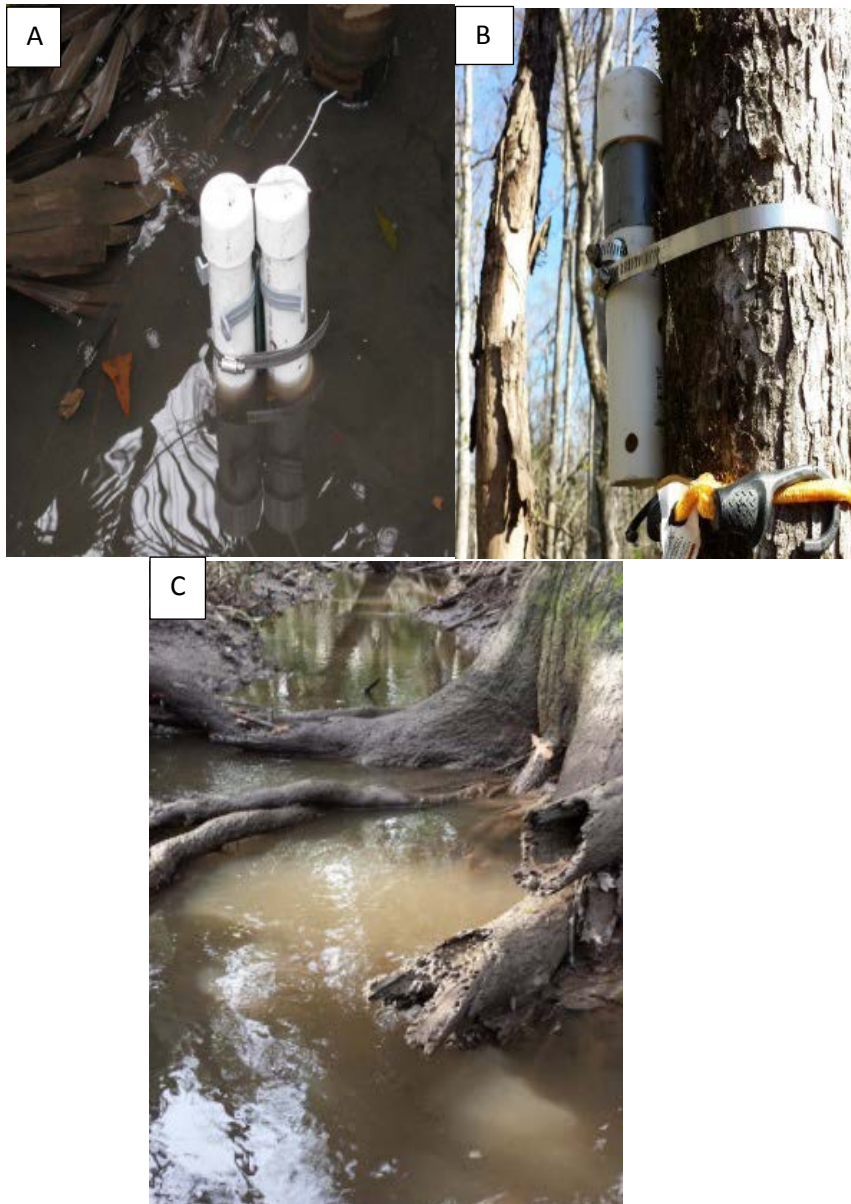
Figure 2. 4: Photographs of (A) conductivity logger and pressure transducer located at site SMR-3 along the St. Marks River, (B) Solinst barometer, and (C) a drainage inlet creek along the East River.
