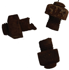
Broken nuts and bolts - remains from when maintenance machinery removed
