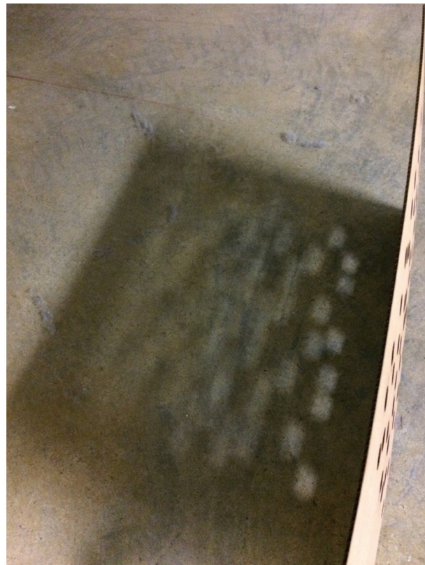
With the same cardboard, same location to make some holes on them, and change one element each time, under the same light, to show the different shadow between them. The shape, size, density of the holes will all affect the effect the shadow.
