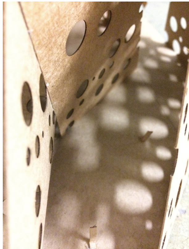
With the same cardboard, same location to make some holes on them, and change one element each time, under the same light, to show the different shadow between them. The shape, size, density of the holes will all affect the effect the shadow.
