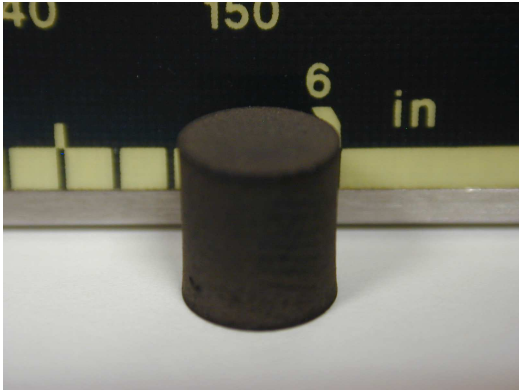
Figure 55 HfC foam created from polymer cylinders
