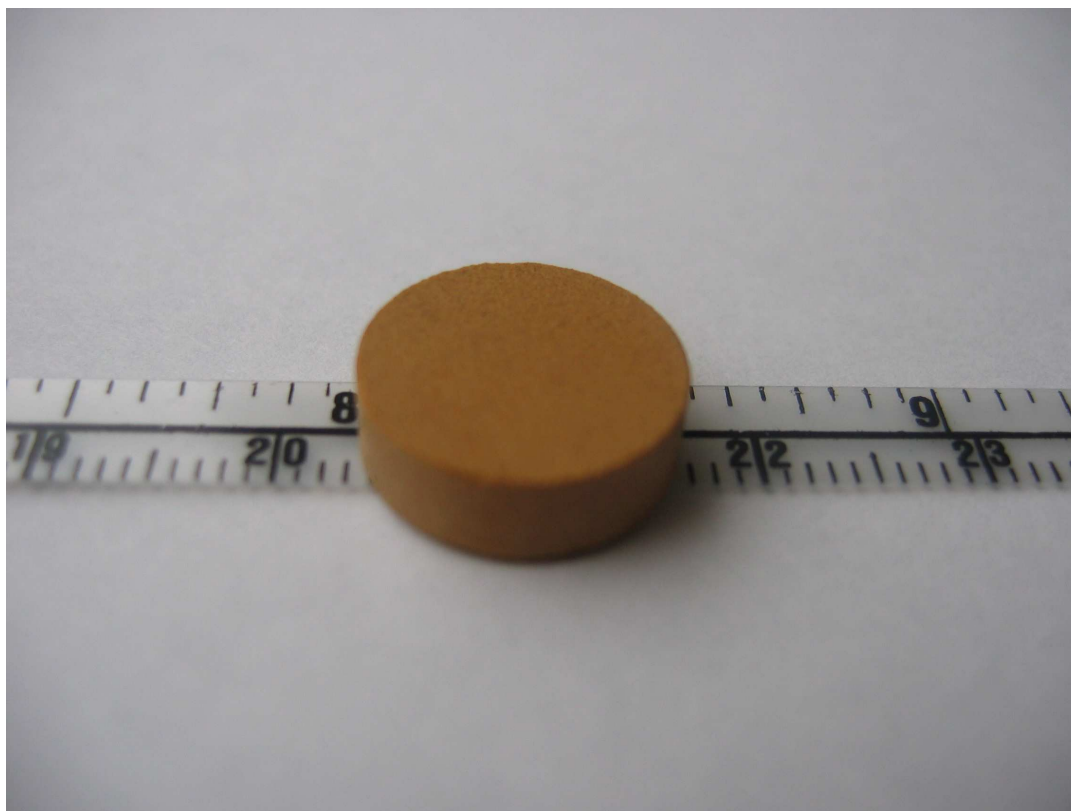
Figure 52 Polymer pellet (cylinder) made from cold pressing of polymer powder
