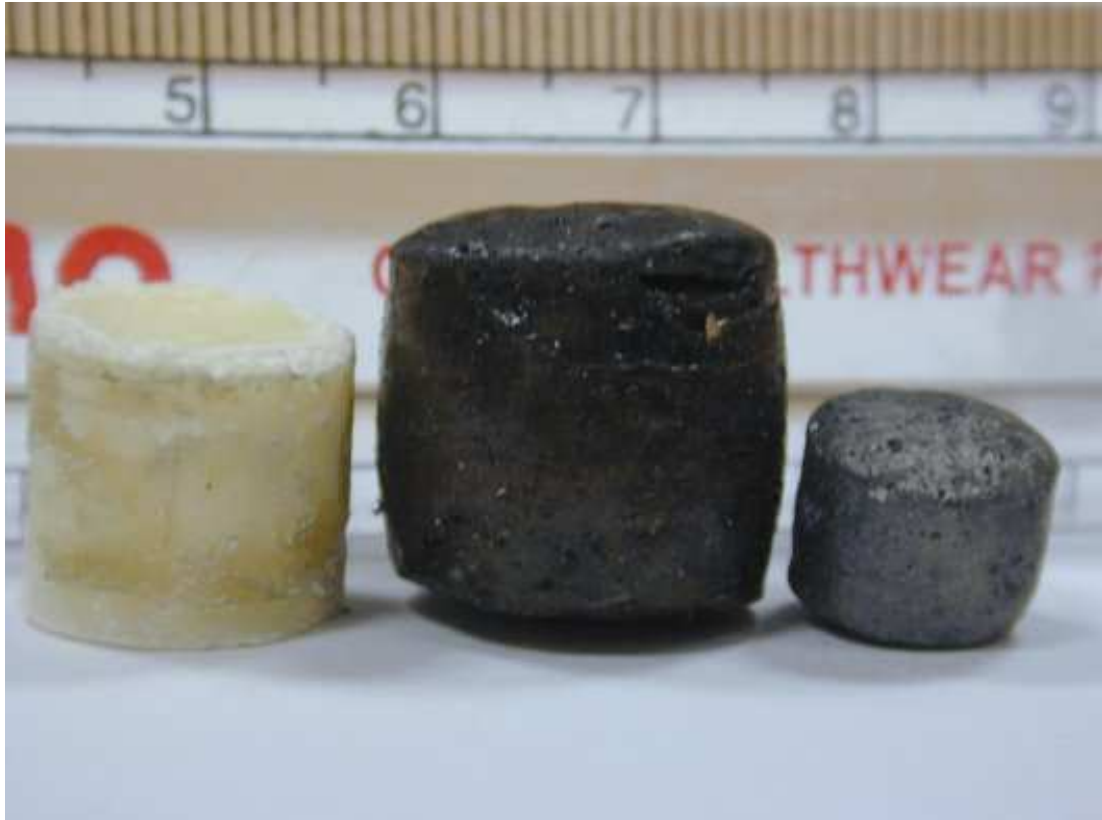
Figure 34 Three different specimens after halting processing at each of the three major steps (from left to right: preform, after thermolysis, after pyrolysis).
