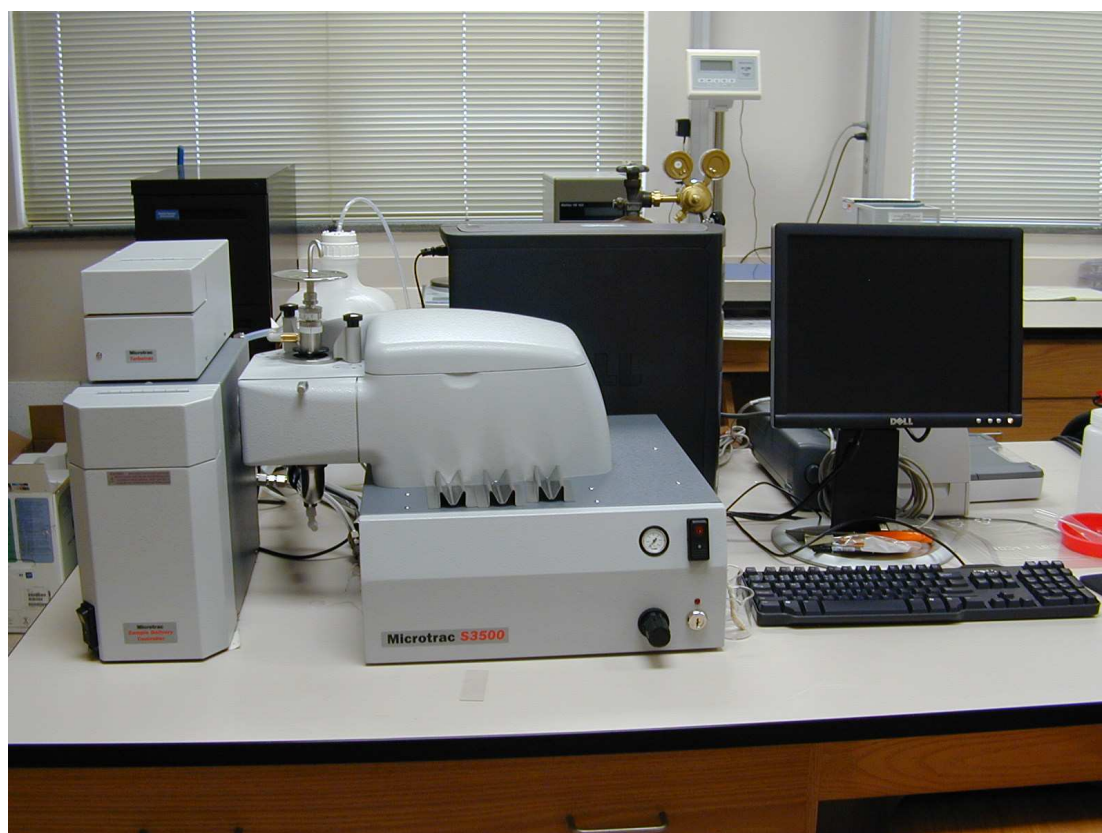
Figure 15 Microtrac S3500 particle size analyzer
