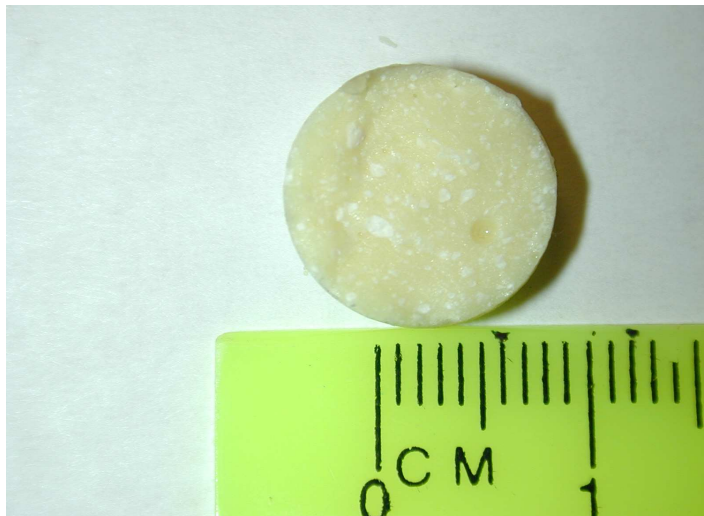
Figure 44 Hand mixed preform sample broken surface (1:1 Mixing ratio). Upper Figure shows entrained air pockets. Lower Figure shows Hf containing agglomerated particles.
