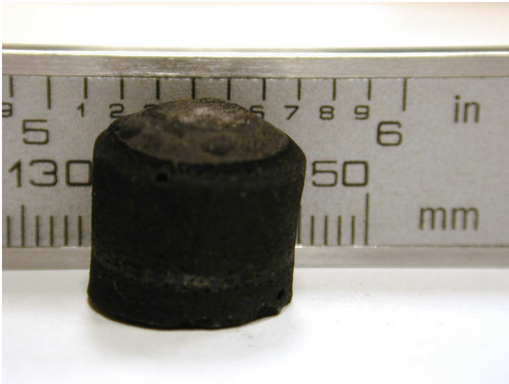
Figure 46 Vacuum mixed HfC foam sample after heat treatment
