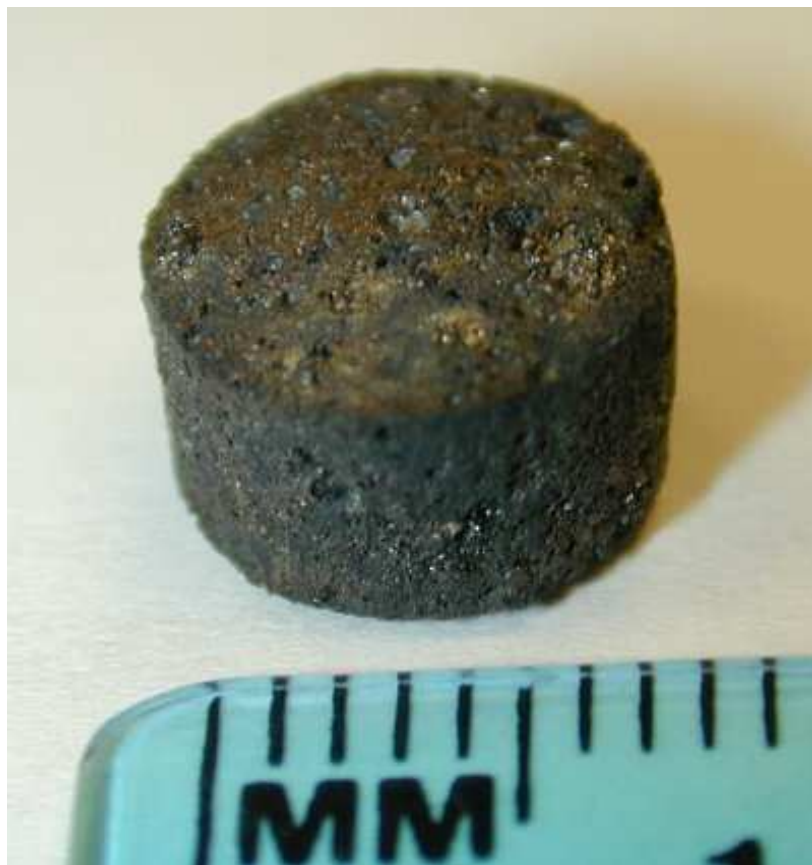
Figure 33 HfC foam (mixing ratio: 3:1) after processing
