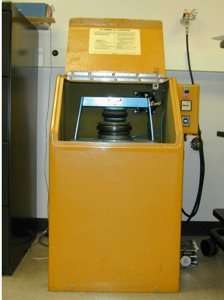
Figure 14 Glen Mills, Labtechnics dish and puck crusher
