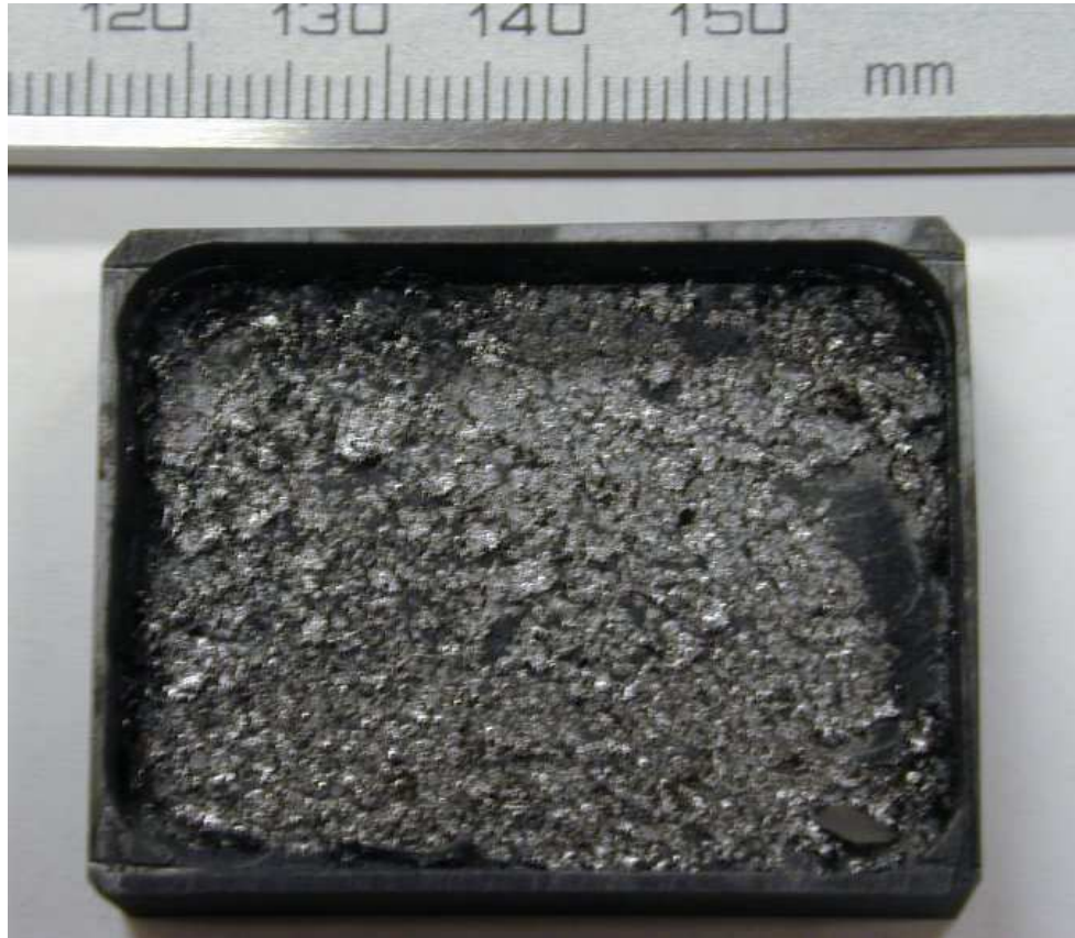
Figure 37 Remains of an epoxy-only specimen exposed to the HfC foam process heat treatment. (Note that the specimen boat was completely filled with hardened epoxy before the heat treatment.)
