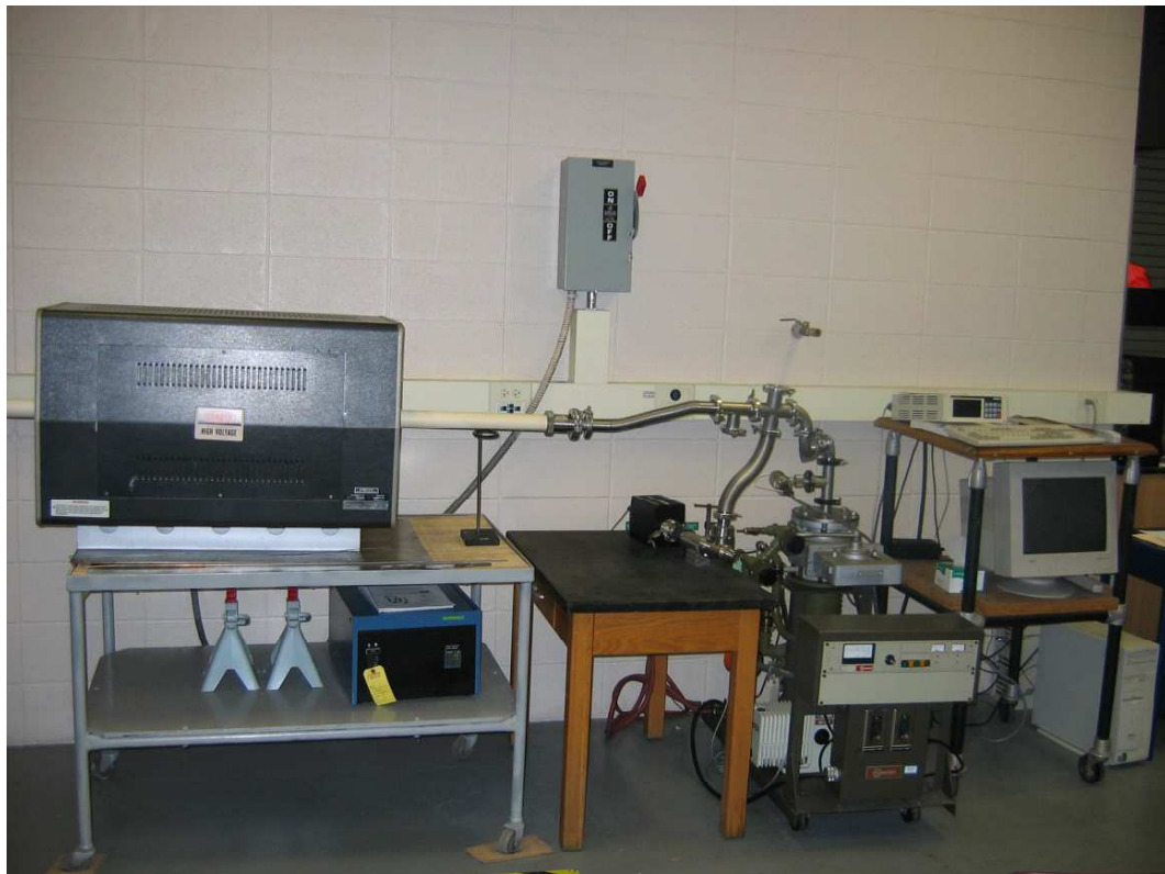
Figure 18 RGA analysis system set-up
