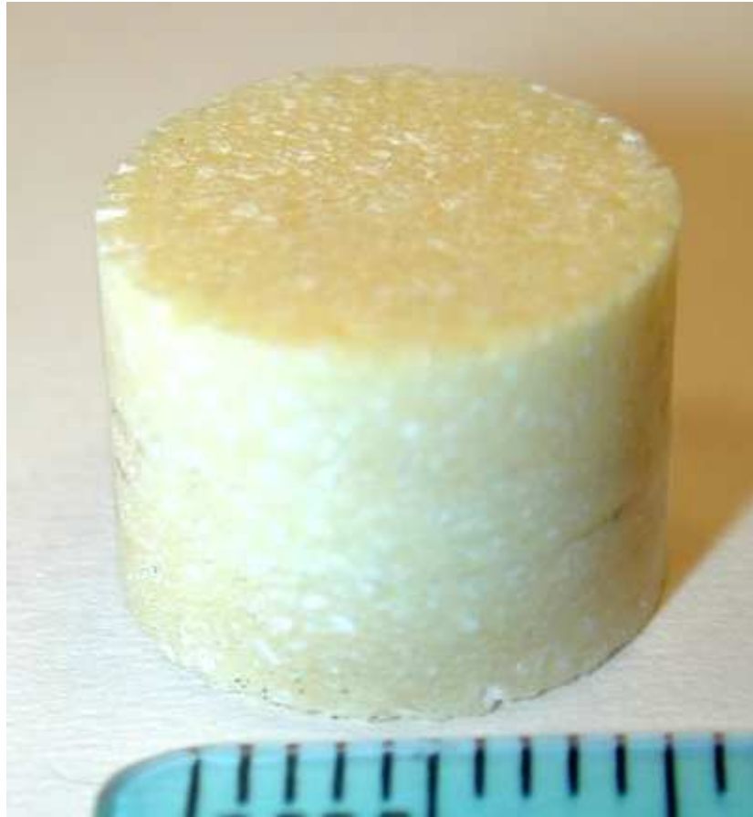
Figure 32 Photograph of preform (mixing ratio: 2:1) before heat treatment
