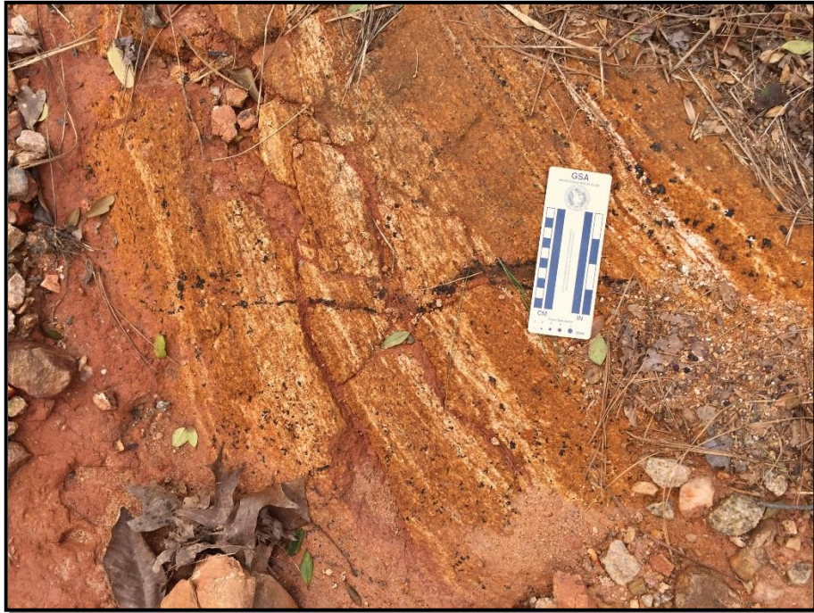
Figure 15: Photograph of weathered banded amphibolite within the Emuckfaw Group, exhibiting the typical porous, punky brick-bat appearance. View is looking northeast ( 33^{\circ}14'10.32'' , -85^{\circ}18'8.28'' ).
