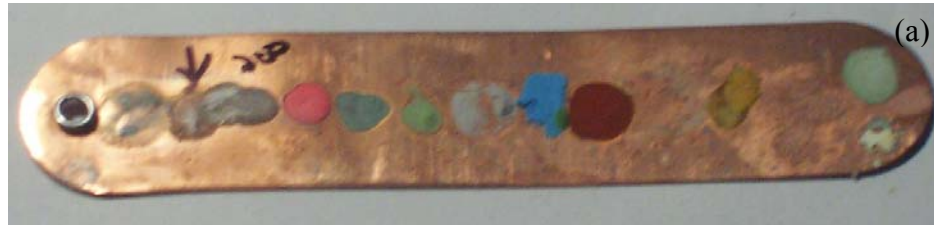
Figure 4.2 Design of the pyrometers(a) and placement (b) during the prescribed fires at the Escambia Experimental Forest.
