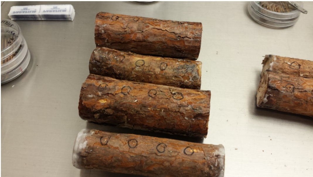
Figure 7.1 Pinus taeda bolts with inoculation holes for inoculation of fungal cultured toothpicks.
