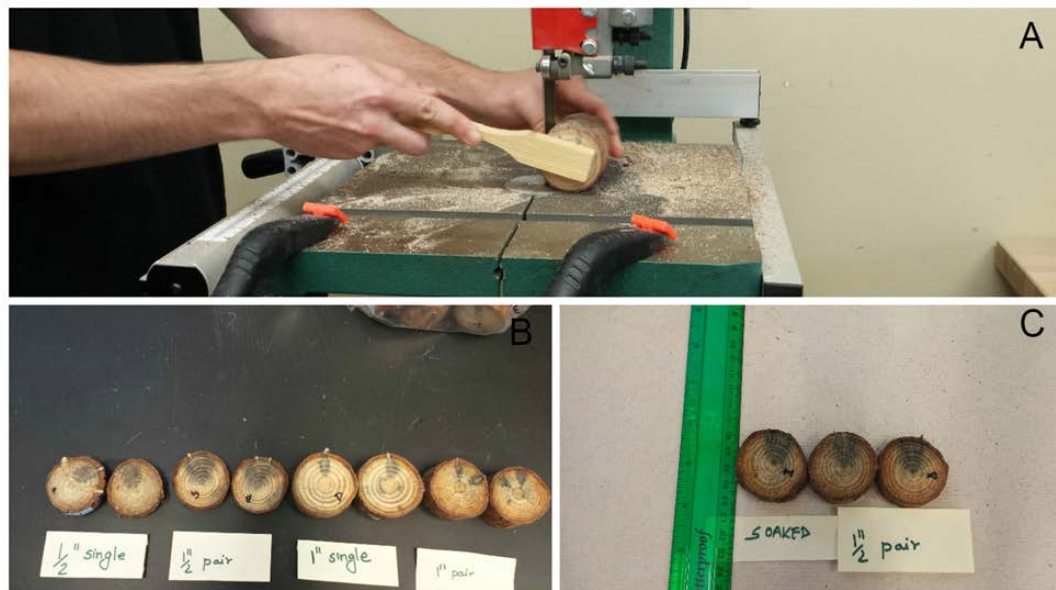
Figure 6.8 A Cutting of the bolts with the band saw B Development of the fungal stain in different treatments C Staining developed in soaked 2.54 cm treatment.
