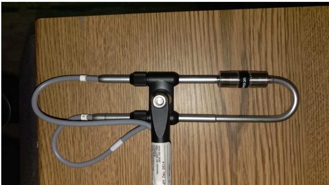
Figure 58: Sound intensity probe with microphones in the face to face arrangement.
