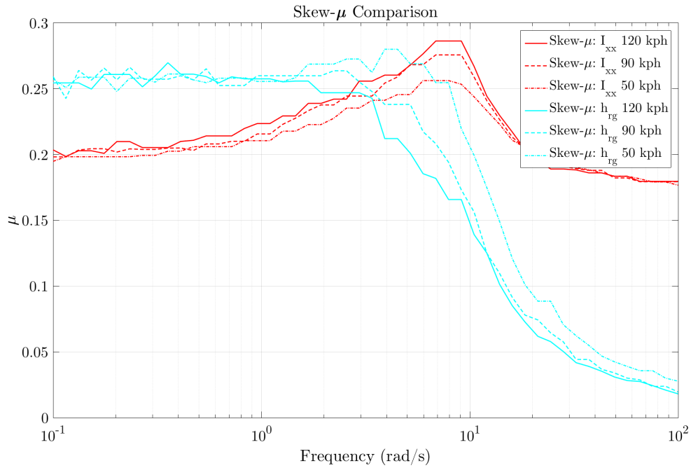
Figure 5.15: Skew \mu of Roll Inertia and c.g. Height with 15% Initial Uncertainty on Each Parameter for Speeds of 50, 90 and 120 kph
