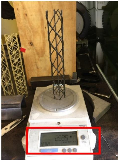
Figure 3.13: OACS Mass measurement for FE modelling
