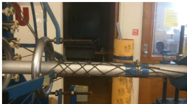
Figure 1.10: Braiding OACS tubes
