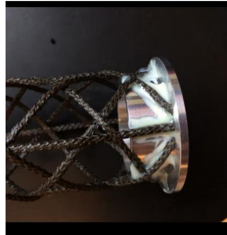
Figure 3.11: Modelling of Aluminum flange - Boundary condition
