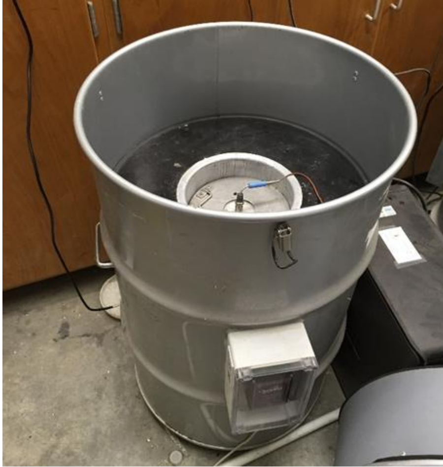
Figure 4-7: Q-Drum testing apparatus
