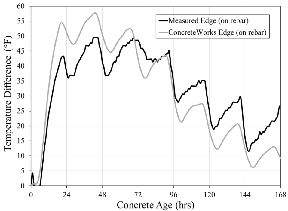
Figure 6-8: Scottsboro bent cap measured temperature difference data versus ConcreteWorks predictions (Eiland 2015)
