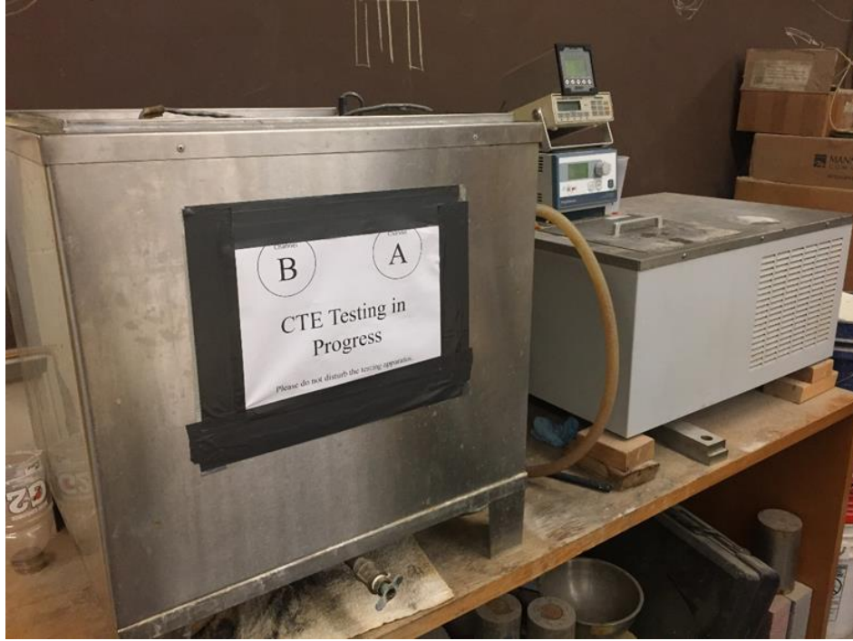
Figure 4-8: CTE testing apparatus
