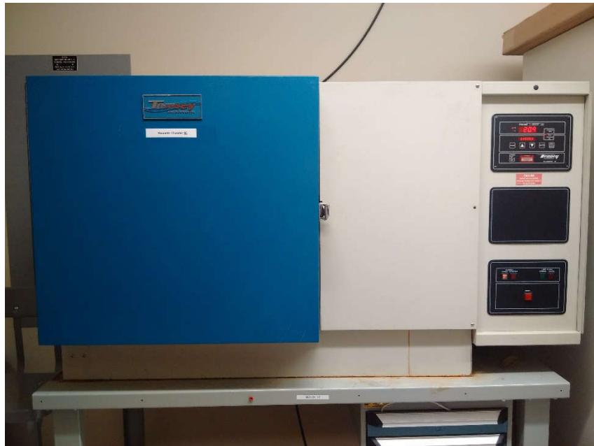
Figure 2.4: Tenney Environmental Humidity/ Temperature System
