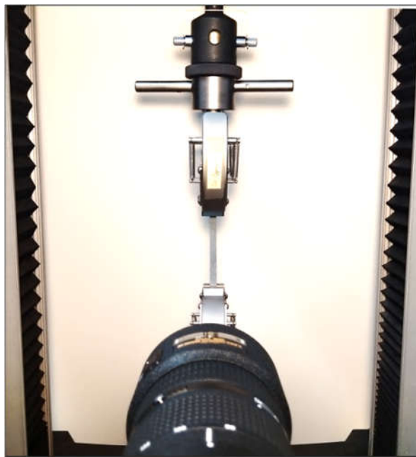
Figure 3.30: DIC Test Setup
