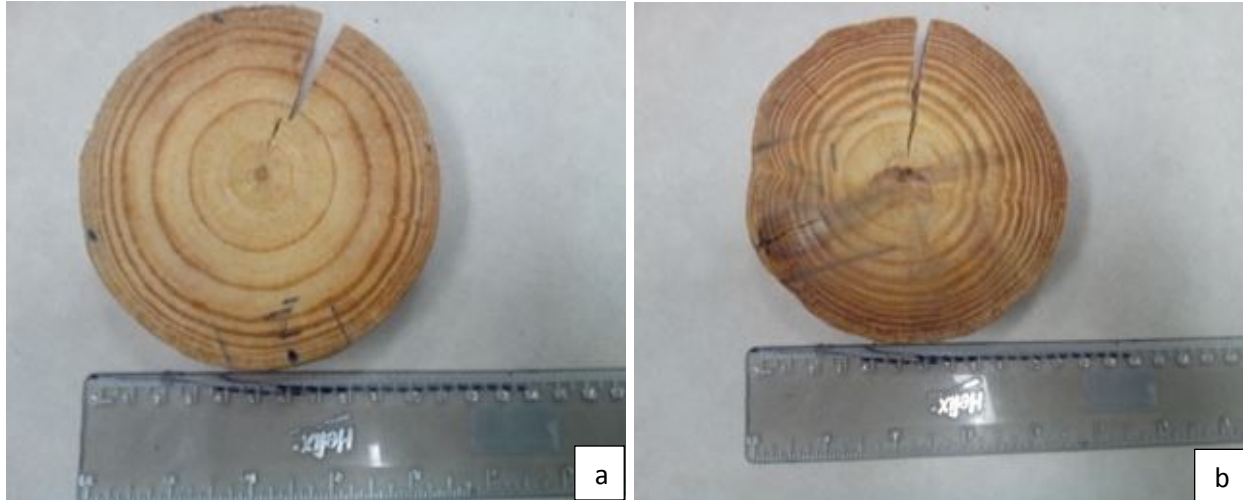
Figure 2.11 Typical growth pattern of (a) normal 14 year old loblolly pine and (b) suppressed 14 year old loblolly pine
