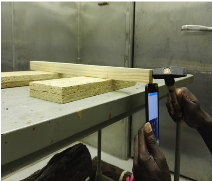
Figure 4.2 Setup for the estimation of acoustic velocity using resonance log grader
