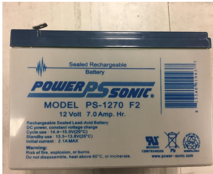
Figure 3.1: 12V Lead Acid Battery
