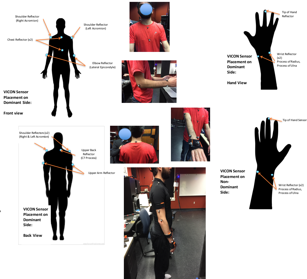
Figure 3.4: Layout of the Reflective Markers Used to Identify Kinematic Segments
