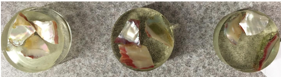
Figure 66. Nacre samples were mounted in a resin. They were grinded into the approximately same height and polished to have a flat and smooth surface.
