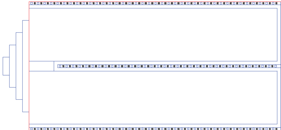
Fig. 3-22 Layout of Integrator Capacitance Cell
