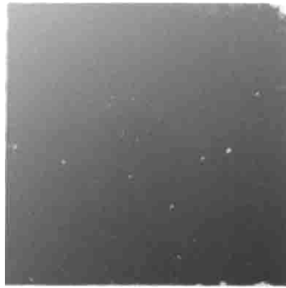
Figure 4.9 Assembly with optimized placement parameters, X-ray image showing only tiny voids
