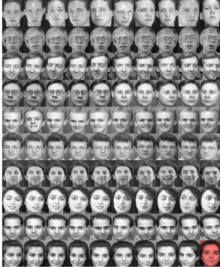
Figure 4.16 Classification result of 100 Olivetti Face data using the presented DDR method with a total processing time of 0.5635 seconds. It shows an impressive classification result and 99% faces are correctly classified. Only one face image marked with red color in the last row is classified as an outlier.
