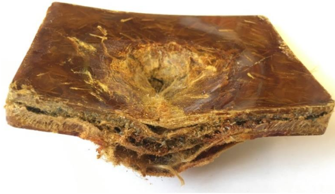
Figure 33: Composite after the drop tower test. Six impacts were needed to penetrate the material with a thickness of 8.5 mm.
