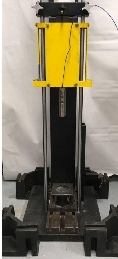
Figure 15: The drop tower test is used to confirm computer simulations and theoretical approaches. Plastic deformations of the test samples can be compared with the computer simulations.
