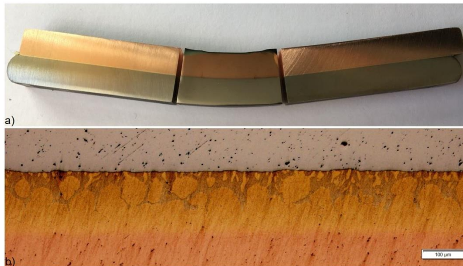
Figure 28: Picture a) shows the deformed composite stripe. In picture b) the brazing joint of the most deformed middle part is examined.
