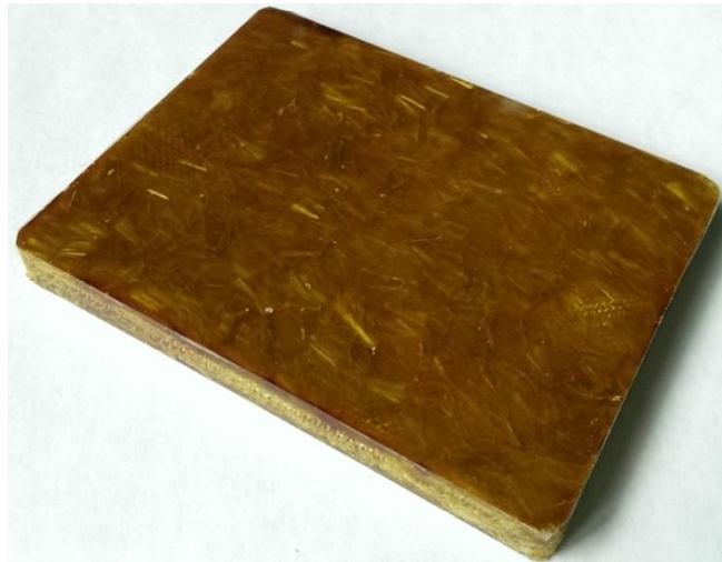
Figure 30: Composite material after the casting. The demonstrated sample has the dimensions of 98 x 75.5 x 7.5 mm.
